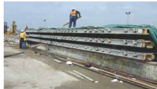
Precast concrete panels on the 24th Street bridge were 8 in. thick, 10 ft long, and 52 ft 4 in. wide. Two panels framed the width of the bridge using a center longitudinal joint. Here panels are shown in the precaster's plant following supplemental steam curing. There were a total of 70 panels on the bridge.
